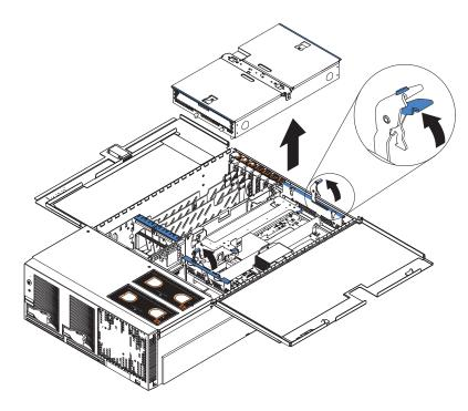
4. Remove the shipping thumbscrews from the right side of the server, and lift the retention bracket from the server.
